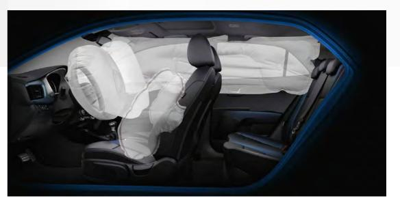
**Six airbags** To help protect occupants and potentially reduce injuries in the event of a collision, the Rio includes front airbags for the driver and front-seat passenger, two airbags at the sides and two curtain airbags running the length of the cabin.
