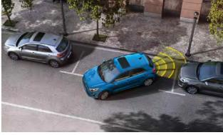
Reverse Parking Distance Warning (PDW) with Switch On/ Switch Off button Ideal for confident parking, PDW uses ultrasonic sensors mounted on the rear bumpers to warn of any obstacles in front or behind when manoeuvring into a parking space. The audible beeps can be switched on or off.
